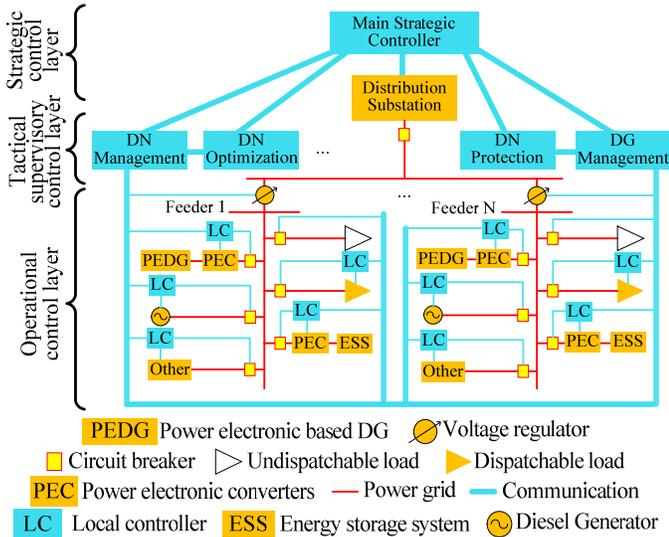
Fig. 3. Illustration of a hybrid hierarchical control framework.
