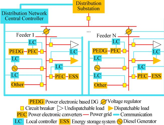
Fig. 1. Illustration of a centralized control framework.
