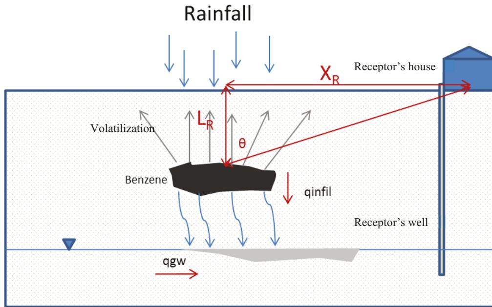
**Figure 2** Conceptual model of contaminant transport, and transport mechanisms ( $X_R$  = horizontal distance between plume and receptor's house,  $L_R$  = vertical distance between plume and surface,  $q_{infil}$  = Infiltration flow rate,  $q_{gw}$  = groundwater flow rate)
