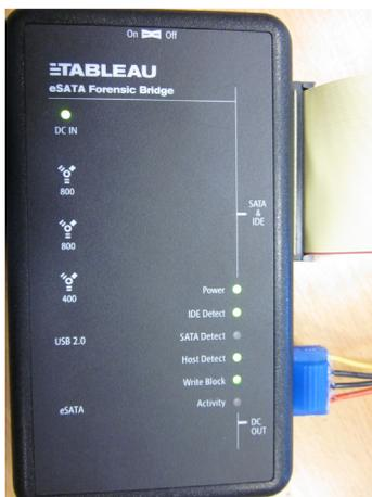
Fig. 1. Hardware write blocker.
